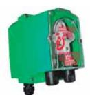
Material: PP. Green. Pump body material: green PP - Peristaltic tube material: silicone -Dimensions: 100 x 80 x 80 mm - Maximum flow: 1 l/h - Maximum -pressure: 4 bar -Connection tube: 4 x 6 mm - Power supply: 230 Vac - 50/60 Hz - Protection : IP 65 Mechanical adjustment -
