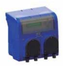
Dimensions: 177 x 171 x 132 mm - Deterg. flow rate: 3-4,5 l/h (1,5 bar) - Rinse aid flow rate: 1,2-2,1/h (2,5 bar) - Power supply: 230 V.
