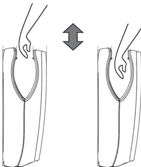
When motor starts, countdown will be shown on the display of the device, which is similar to a barcode. The optimal drying time would be one cycle of the barcode display. However if the user wishes to continue with the drying, another cycle will start automatically without being necessary to remove hands and introduce them again. Maximum drying time is 30 seconds.
